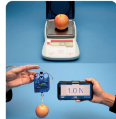
Figure 32.15 This apple has a mass of 100 g and a weight of 1 newton.
