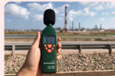
Figure 41.1 A sound-level meter is used to compare the loudness of different sounds.
