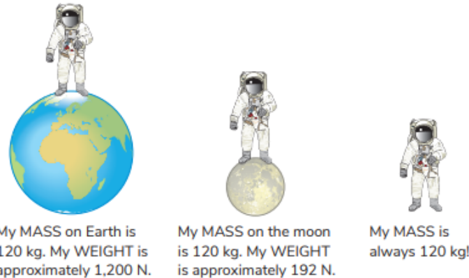
Figure 32.14 The weight of a body will change depending on location. The mass will not change just by moving it.
