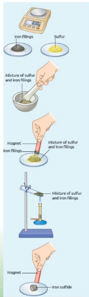
Figure 17.8 Investigating the properties of a mixture of iron and sulfur and of the compound iron sulfide
